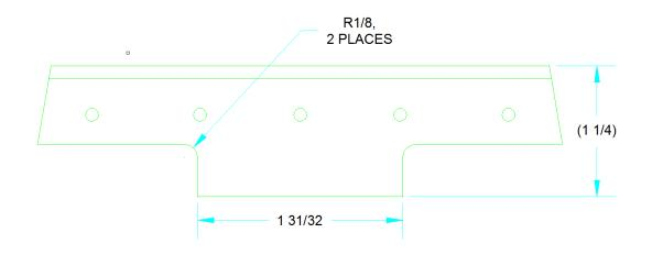
FIGURE 3: MODIFIED UP ELEVATOR STOP TOP VIEW
